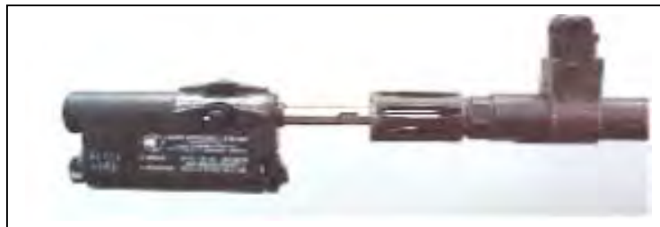
Figure G-3. Bore light in the HALF-TURN position.
